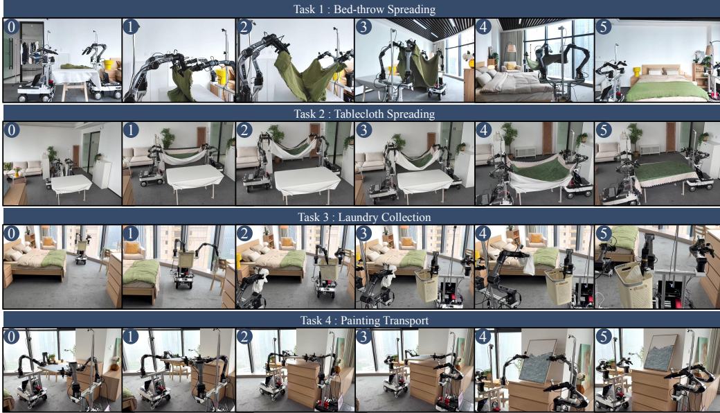
Figure 3: Real-world task suite. Representative rollouts across deformable spreading, shared-workspace collection, and rigid-object transport.
