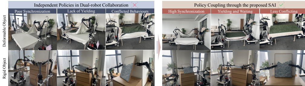
Figure 1: Local skills are not enough for dual-robot coordination. Independent policies can fail under phase mismatch, insufficient yielding, and physical interaction conflict. SAI induces coupled behavior.
