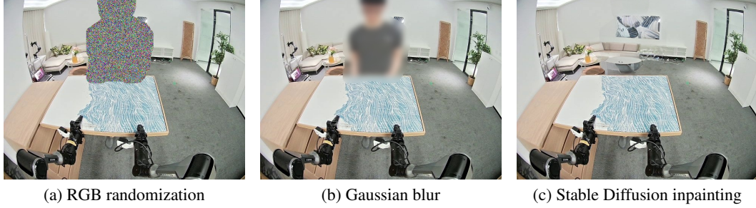
Figure 6: Partner-region randomization. Training-time replacements applied inside the detected human-partner region: RGB randomization, Gaussian blur, and Stable Diffusion Inpainting.
